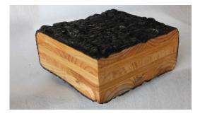
Figure 1 CLT that survived a complete burnout of a structure showing the protective char layer from (XLam, 2017)
